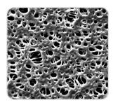
Polyethersulfone (PES) membrane filters are hydrophilic, have high flow rates, a low non-specific protein adsorption and are chemically resistant over a pH range of 1 – 14. They are therefore recommended
