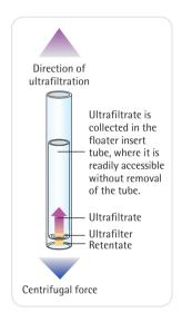
Centrisart<sup>®</sup> I\* is a ready-to-use unit for small-volume, centrifugal ultrafiltration to separate proteins from low molecular weight substances in biological samples.
