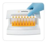
Close the station lid. The grooves align the caps automatically, securely sealing every single Claristep® Filter unit for the most convenient processing.
