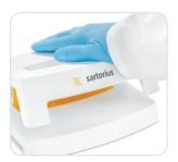
2. Apply slight uniform pressure with your hand to start sample clarification. You will feel a certain resistance while liquid is pressed through each membrane.
