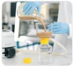
2. Mix to homogenize. Pour the cell culture and filter aid mixture into the Sartolab® RF first ...
