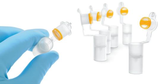
Claristep® Filter units are made of the purest materials. Another major benefit is that the contact time of the samples with the filters and the caps is extremely short, ensuring optimal, contamination–free results. Filtered liquids are collected in any 12 × 32 mm outer diameter vials of your choice based on the analytical method to be performed.
