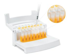
Before clarification, the samples are pipetted in the filter reservoire.
