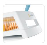
Claristep® Filter units press liquid through each membrane by an air pocket that forms over each filter unit when the station lid is closed. This air pocket is released when you stop holding down the lid – you will feel it in your fingertips!
