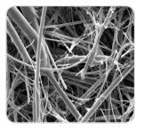
These filters are mostly used either for monitoring air and gas or as a prefilter. They are manufactured with synthetic binding agents to ensure that the filter has a defined strength.
