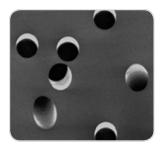
Those white and hydrophilic polycarbonate track-etched membranes are manufactured from high grade polycarbonate film using track-etch technology. Their capillary pore structure is uniform and precise, with a narrow pore size distribution to retain particles on their surface. Track-etched membranes are an excellent choice for accurate fractionation of particulates because of their precise pore size.
