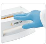
**3.** Press down on the station lid so that the left and right corners touch the base plate. Hold the lid in place for 3 seconds to ensure all sample liquid is filtered through.
