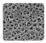
The very low adsorption membranes are hydrophilic, solvent-resistant (pH 3-12) and therefore suited for the particle removal from solvents. The membrane is reinforced with nonwoven cellulose. They are available in two pore sizes:  $0.45 \mu m$  and  $0.2 \mu m$ .
