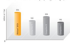
0.45 µm SFCA membrane compared with CA (Cellulose Acetate) or similar hydrophilic membranes of the same pore size
