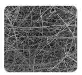
The quartz microfiber material of the Sartorius pre-heated filters, grade Q3400, is made of high-purity quartz microfibers without any addition of glass microfibers or binding agents. In addition, the Q3400 filter grade is tempered to remove all chemically combined water and to give the filters
