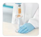
**3.** Connect the sterile filter to the syringe and filter.
