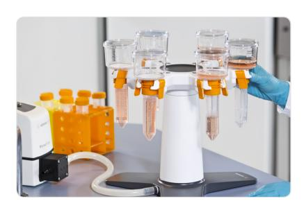
The MultiStation advantage: Using the Sartolab® MultiStation to filter 6 x 50 mL samples saves handling time compared to standalone filtration
