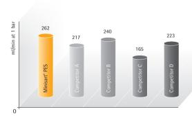
0.45 µm PES membrane compared with other PES membranes of the same pore size
