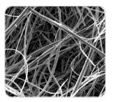
Binder-free glass microfiber filters are recommended for analytical and gravimetric analyses and also as prefilters. These filters combine fast flow rates with high load capacity and the retention of very fine
