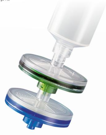
Non-presterilized Minisart® units: High Flow, NML, NML Plus and HY can be sterilized by ethylene oxide; High Flow, NML and NML Plus can also be sterilized by gamma irradiation
