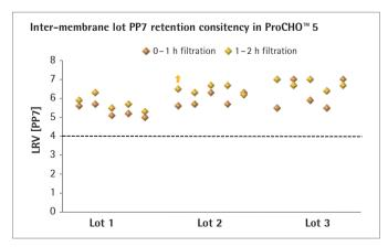
Figure 7: Inter-lot PP7 retention consistency in  $ProCHO^{\text{m}}$  5 cell culture media. Absolute retention is indicated by the arrow.
