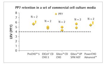
Figure 4: PP7 retention in a set of commercial cell culture media. Absolute retention is indicated by the arrow
