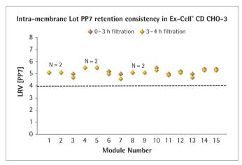
Figure 6: Intra-membrane lot PP7 retention consistency in ExCell  $^{\circ}$  CD CHO-3 cell culture media
