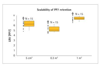
Figure 8: Scalability of PP7 retention over the whole product family of Virosart® Media. Absolute retention is indicated by the arrow.
