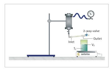
Figure 1: Experimental set–up for spiking study using Virosart $^{\circ}$  Media lab module 5 cm $^2$
