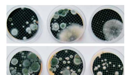
It generally proves practical to place petri dishes with agar or with moistened nutrient pads plus a membrane filter, directly in the filling room and to leave them exposed there for several hours – for instance during a filling shift. This offers a direct correlation to the bacterial load that the filling heads are exposed to. As can be clearly seen from the adjacent images, the bacterial load can vary greatly.
