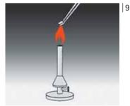
in the filter funnel. The membrane filters are positioned and removed using forceps (8), which must also be sterilized by flaming (9) after each use.
