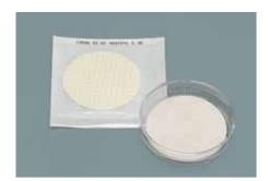
Nutrient pad set with membrane filter
