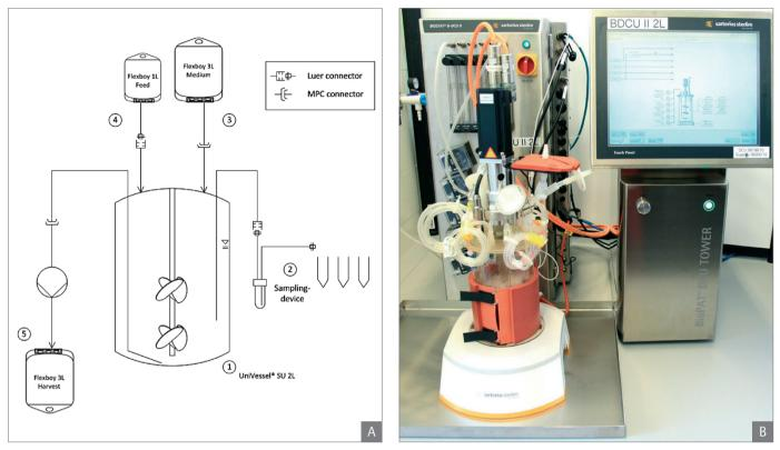
**Figure 1:** Experimental setup of the cultivation process in the UniVessel<sup>®</sup> SU 2L. A) Schematic overview of the experimental setup. The UniVessel<sup>®</sup> SU 2L (1) is additionally equipped with a sampling device (2), medium bag for medium feed after cell attachment (3), feeding bag for partial media exchange on day 4 (4), and harvest bag for cell harvest on day 7 (5). B) Experimental setup at the Zurich University of Applied Sciences (ZHAW).
